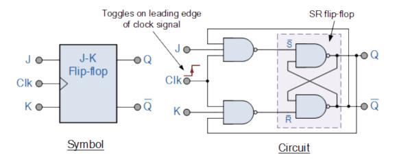
Both the S and the R inputs of the previous SR bistable have now been replaced by two inputs called the J and K inputs, respectively after its inventor Jack Kilby. Then this equates to: J = S and K = R.
